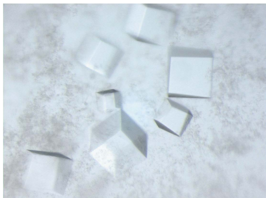
Figure 2 Crystals of Hyb-24 obtained using a reservoir solution consisting of 2.0 M ammonium sulfate, 0.2 M lithium sulfate, 0.1 M MES buffer pH 6.5 and 15% glycerol.
